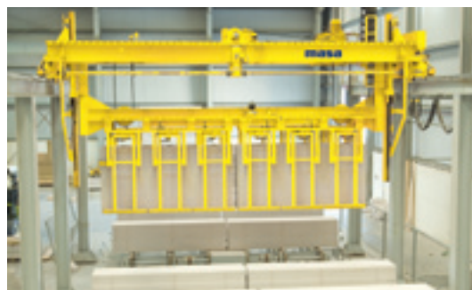
Block shifting device for reinforced panels
