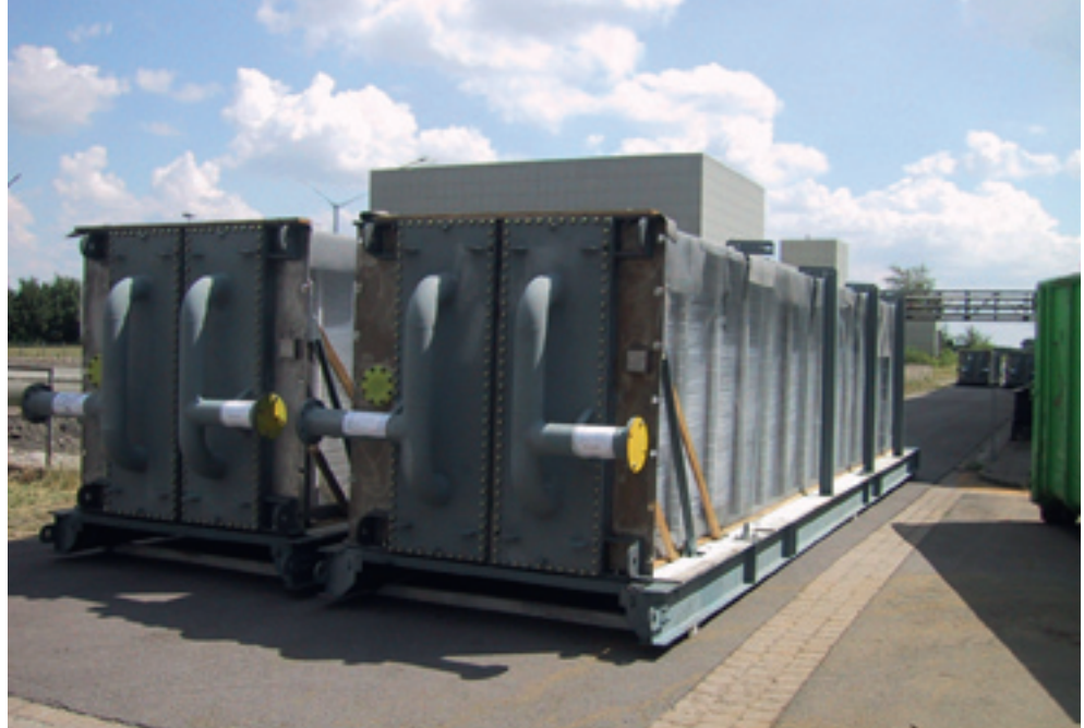
Delivered and stored flue gas cooler modules
